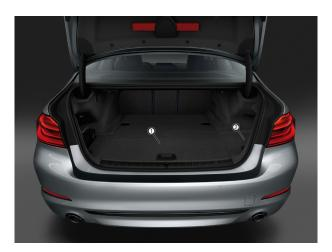
Disconnect the battery earth lead (1, 2) and pull it off toward the top.
