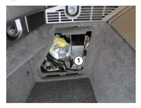
Cut through the cable (1) for the high voltage disconnect (cut solution). The high-voltage system is deactivated.
