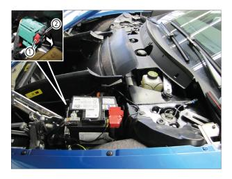
The high-voltage system is deactivated when bore hole (1) is completely free.
